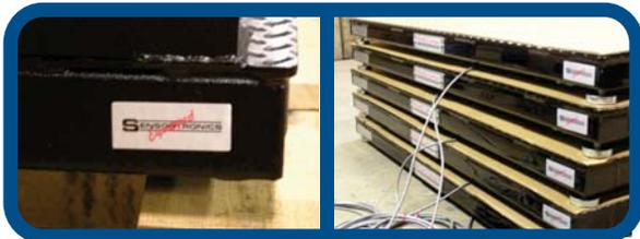
'SENSORTRONICS Equipped' - Thanks to a new commitment from Vishay Transducers, we are using more Sensortronics 65023 load cells in our M6600 series Floor Scales than ever. Our standard floor scale has a 3" nominal height (base of foot to top of deckplate) and is 100% consistent with older units. In fact, we've standardized on the 10K frame for all capacities 1/2/5/10K- true HEAVY DUTY construction and quality components make our 6600 series a tremendous value.
